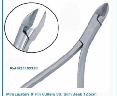
Fitted With Immuunity-HS Steel Tips Insert, Bea Length 8mm, Diamond honed edges, Box Joint. 1/3 Handle Gold Platted. Stainless Steel.
