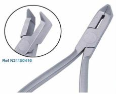
Pliers for forming and cinching round or rectangular wire up to .028". Serrated tips are tapered to a fine point allowing access to difficult reach areas. Rivet Joint. Stainless Steel
