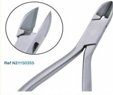
Ligature Cutters Str, Light Slim Model, 7 degree 12cm. Fitted With Immunity-HS Steel Tips Insert, Beak Length 10mm, Diamond honed edges, Box Joint. Stainless Steel.
