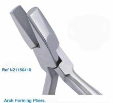
Ideal Plier to create a smooth arch on both round wires up to .040" and rectangular wires up to .021" x .028". Beveled edges eliminate the nicking of the wire during operation. Rivet Joint. Stainless Steel.
